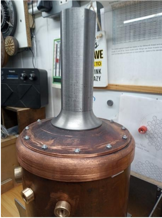
Photo 7 (above left) The finished dome is mounted on a smoke-box top ring of copper that sits over the barrel. The chimney base was machined separately from the chimney and screw-cut 1 1/2" x 32 so the chimney screws into it. Photo 8 (above right) The barrel with bushes in place
