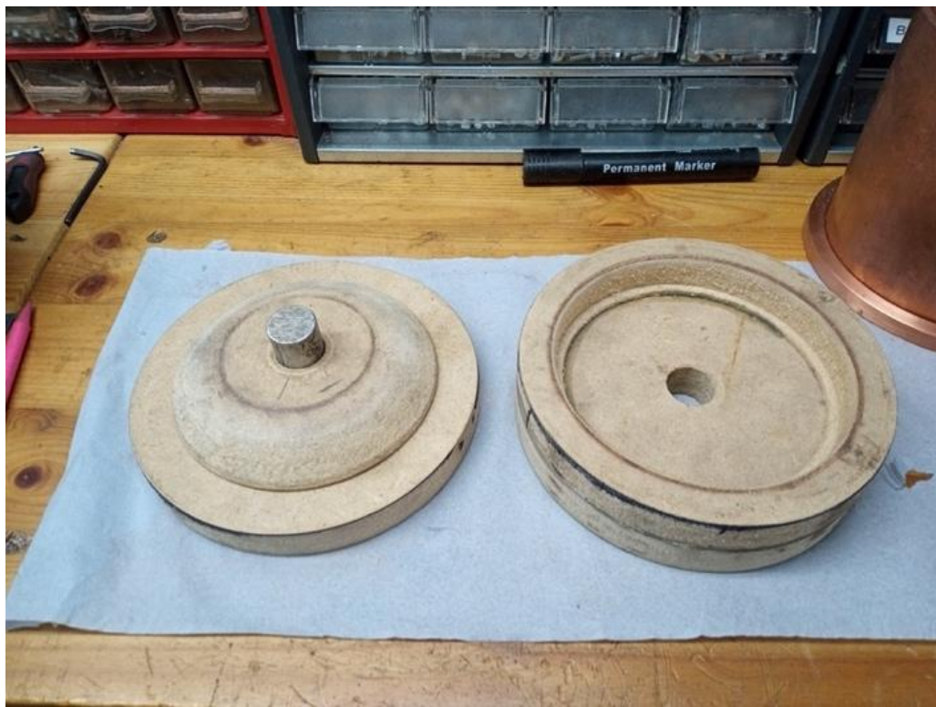
Photo 6 The punch and die were machined from MDF to create the 3mm thick copper dome, pressed between the punch and die with a vice and clamps. It was annealed four times to get the finished product
