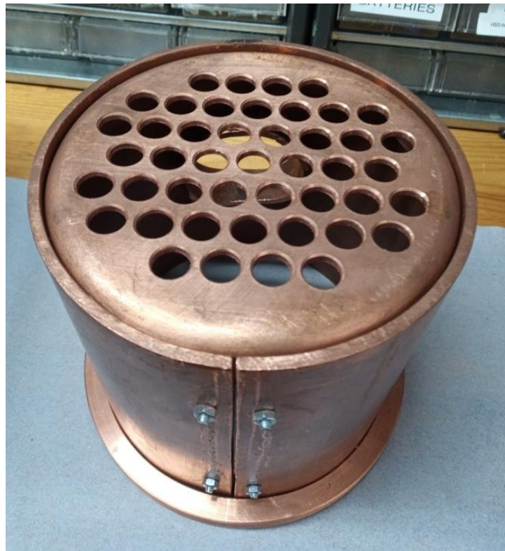
Photo 3 shows the firebox tube plate inserted into the firebox
