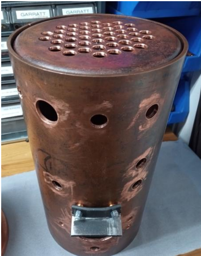
Photo 4 & 5 show the main barrel with the smoke-box tube-plate inserted. It is 6" diameter and 11" long, rolled with a 30mm butt strap. Holes are drilled for bushes for fittings and mounting brackets
