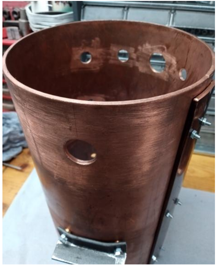
Photo 4 & 5 show the main barrel with the smoke-box tube-plate inserted. It is 6" diameter and 11" long, rolled with a 30mm butt strap. Holes are drilled for bushes for fittings and mounting brackets
