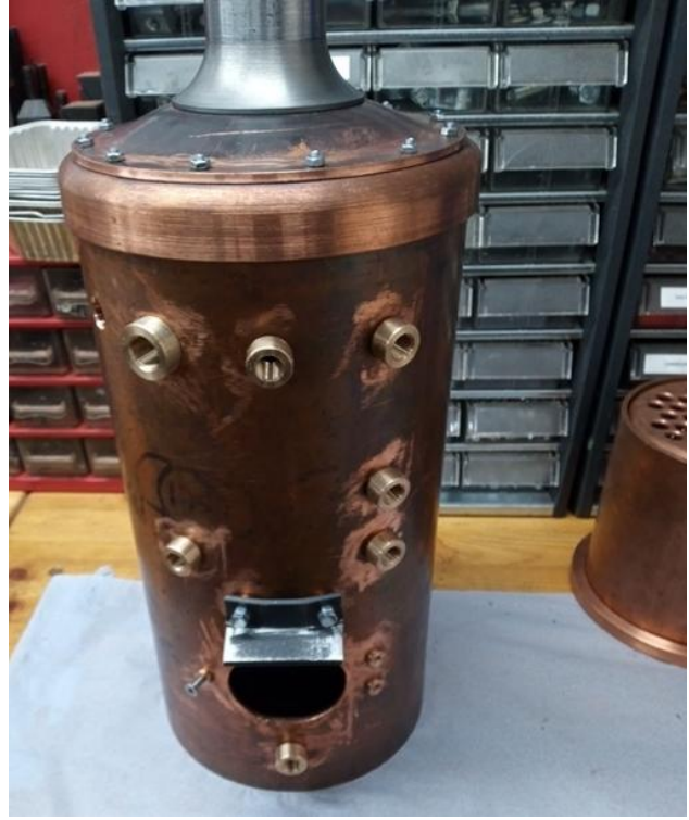
Photo 7 (above left) The finished dome is mounted on a smoke-box top ring of copper that sits over the barrel. The chimney base was machined separately from the chimney and screw-cut 1 1/2" x 32 so the chimney screws into it. Photo 8 (above right) The barrel with bushes in place
