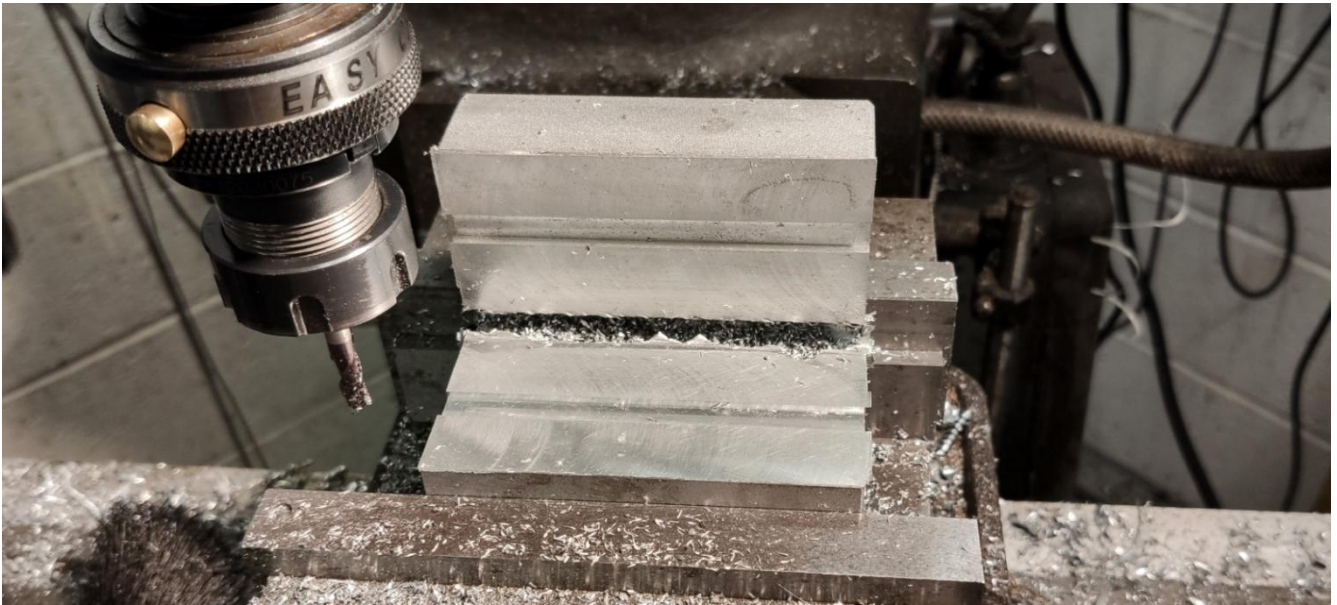
Machining the magnet slot
