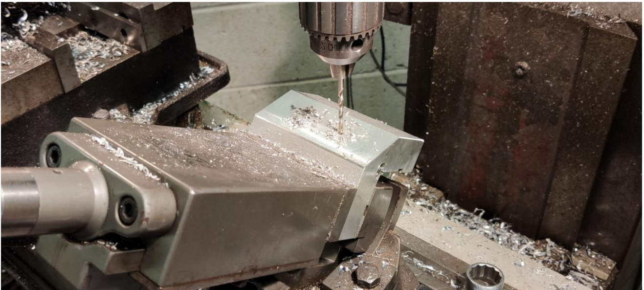
Drilling the securing holes
