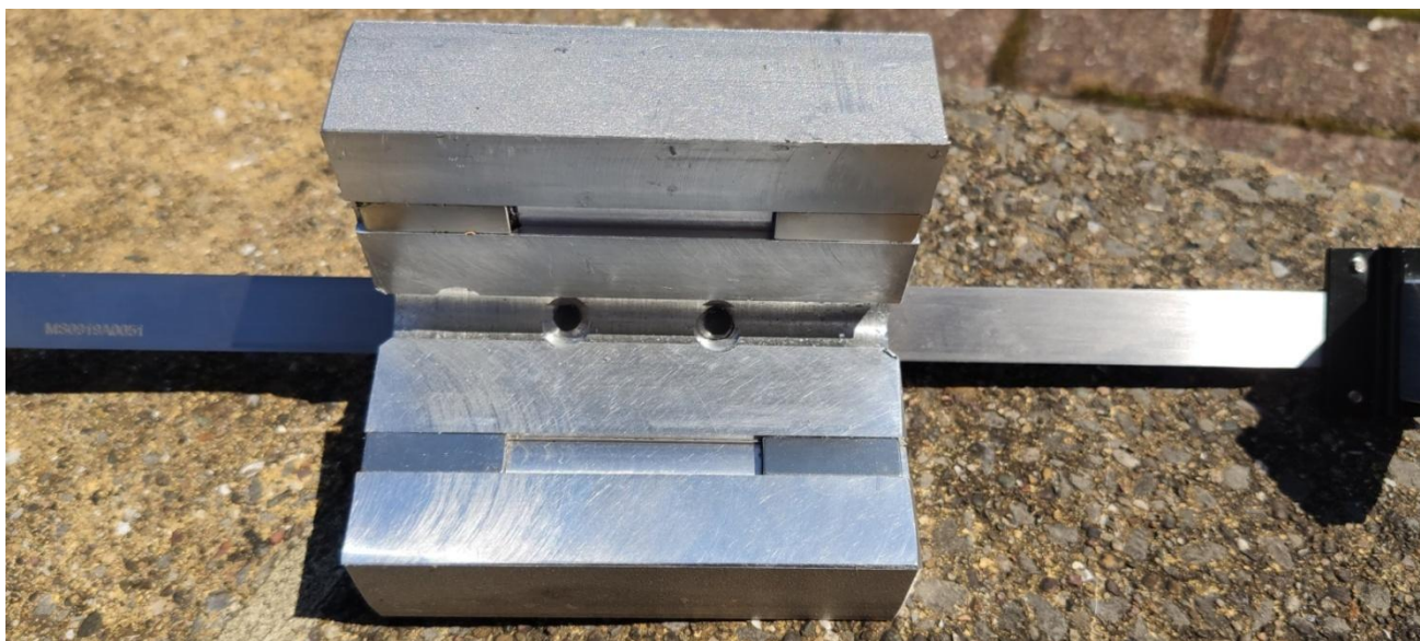
Magnets secured into the slots
