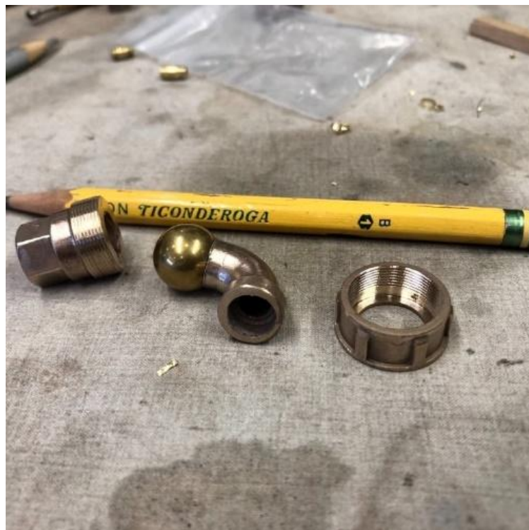
Fabrication of the flexible ball joints
