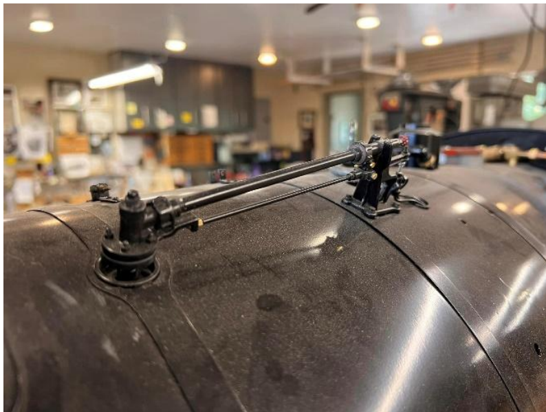
A fabricated Oakadee quick-disconnect water coupling and below the low water alarm.
