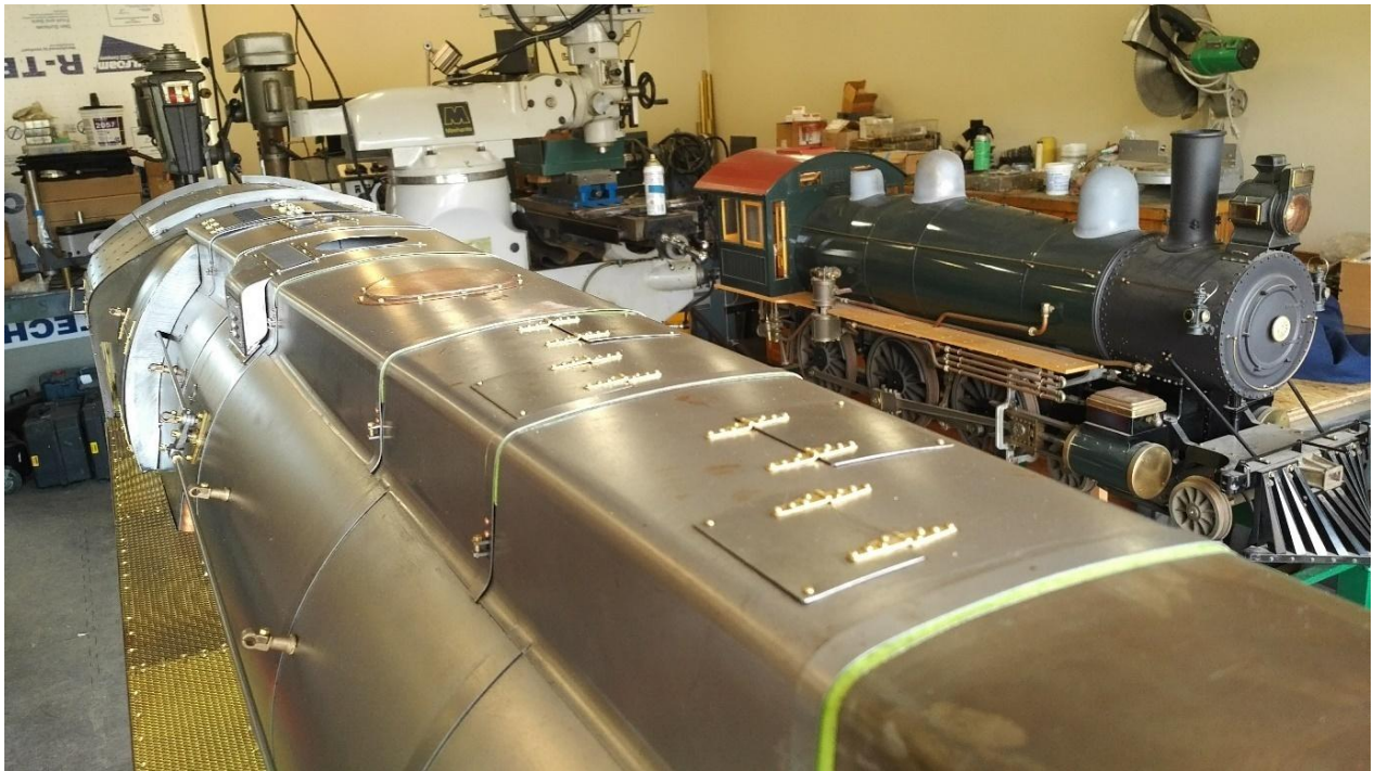
Detail work on the Hudson casing
