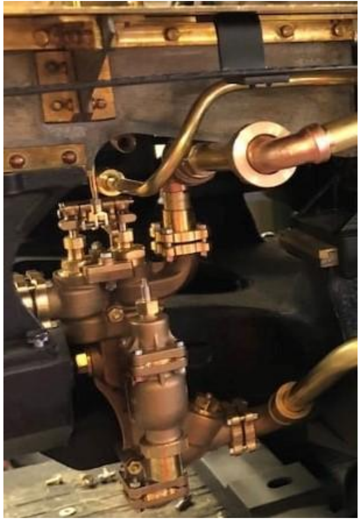
Injector with Barco flexible joints
